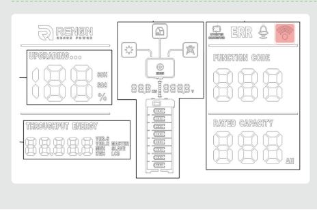
After completing the steps, the WiFi icon on the battery screen will blink, indicating it's connected to the router. Then, set the inverter code to "000000".
