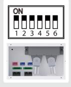
Set the inverter dial code (INV SET) to all up (111111) as shown above before proceeding with Wi-Fi setup.
