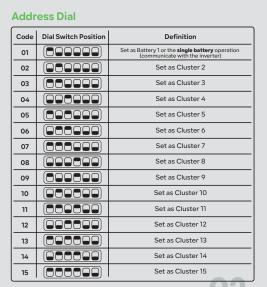
Set the dial codes sequentially for each battery when connected in parallel, supporting up to **15 units.**
