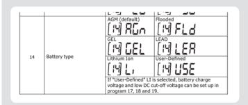
After pressing and holding "ENTER" button for 2 seconds, the unit will enter setting mode. Press"UP"or "DOWN" button to select setting programs 14 to "Lithium Ion" battery type , And then, press "ENTER" or "MENU" button toconfirm the selection and exit.
